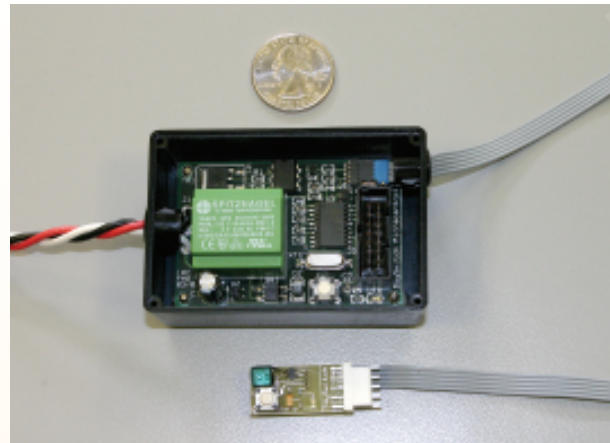
The DaySwitch consists of a microcontroller (top) that switches the luminaire on and off, and a photosensor (bottom) that measures daylight levels and sends a signal to the microcontroller.
