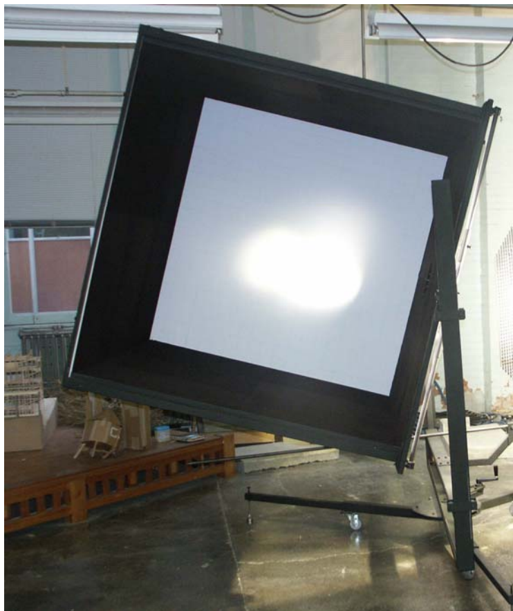
Fig. 3: Configuration to avoid interreflections: one white panel and four black panels
