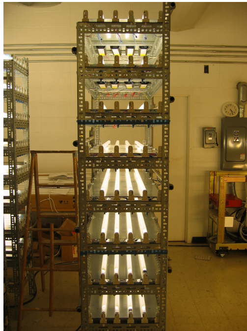
Figure 10. Instant start fluorescent lamp life test rack
