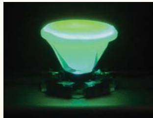
Above: An SPE LED package with a green phosphor when excited by a blue LED excitation light source. Right: An electric laboratory furnace anneals phosphors to temperatures up to 1200°C.
