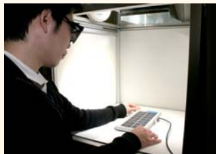
LRC researchers tested PV panels under the standard testing condition of one sun level, 1000 w/m 2 , and verified that the results met the manufacturers' claims.
